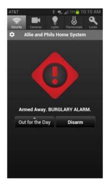
To cancel the alarm and stop the security system's alarm sound, tap the **Disarm** button.
