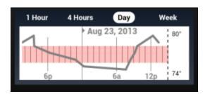
If the temperature goes above the thermostat's cool setpoint, a blue area on the graph indicates when the air conditioner was activated. If the temperature goes below the thermostat's heat setpoint, a red area on the graph indicates when the heat was activated.
