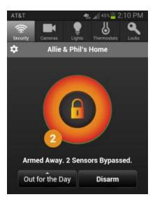
CAUTION: When you bypass a sensor during arming, that sensor no longer provides protection while the system is armed. Using the example above, if you tap Arm Anyway, anyone can open or close the bypassed window while the system is armed without setting off an alarm. Be cautious if you decide to use this feature, because it essentially defeats the purpose of your security system.
